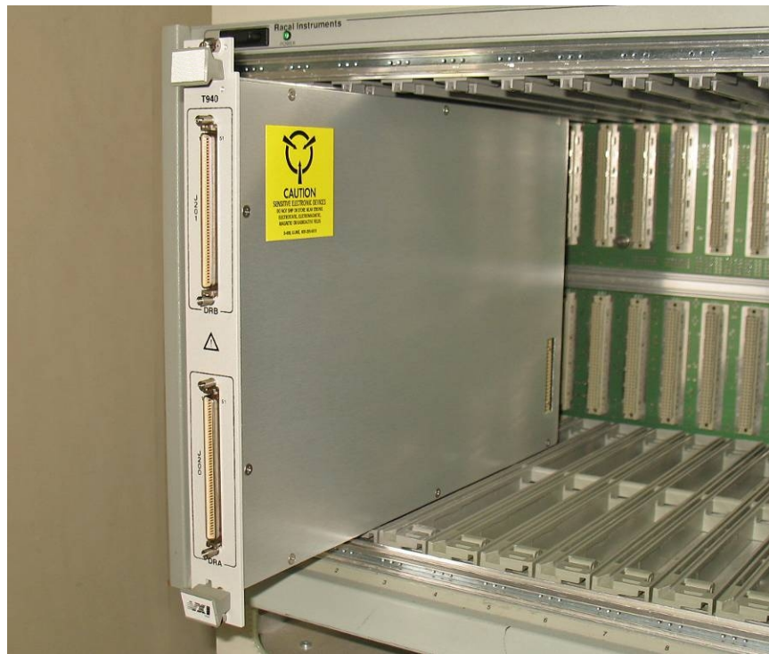
Figure 2-6: Installing the DRM into a Chassis
