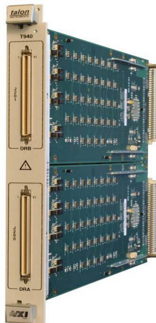
Figure 2-1: T940 with Two DR7 Boards Installed
